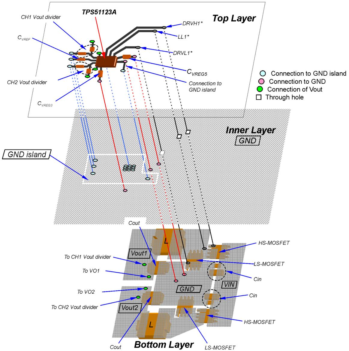
Figure 38. PCB Layout
