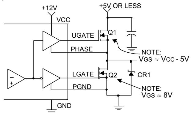
Figure 15. Upper Gate Drive-direct  $V_{CC}$  Drive
