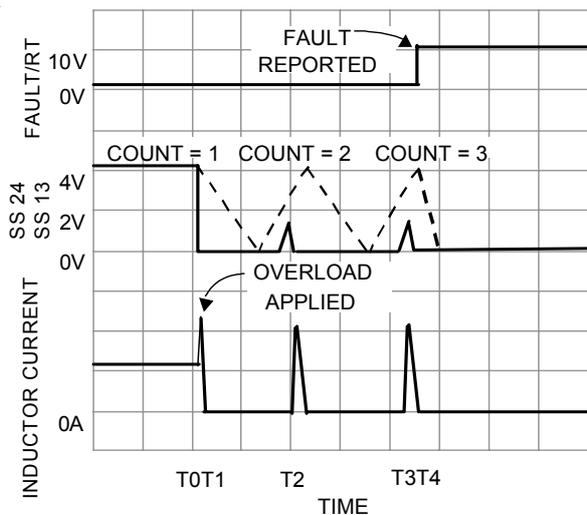
Figure 5. Over-current Operation
