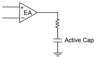
Figure 8. Error Amplifier Compensation
