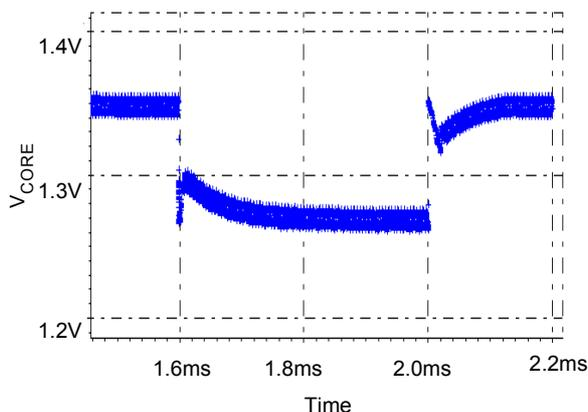
Figure 14.  $V_{CORE}$  Wave Form at Load Transient
