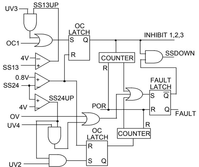
Figure 4. Fault Logic-simplified Schematic
