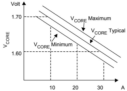
Figure 11. V<sub>CORE</sub> Load Line
