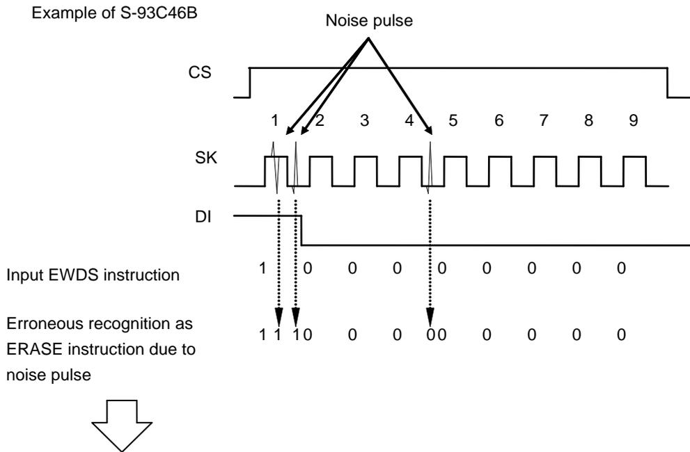
In products that do not include a clock pulse monitoring circuit, FFFF is mistakenly written on address 00h. However the S-93C46B detects the overcount and cancels the instruction without performing a write operation.
