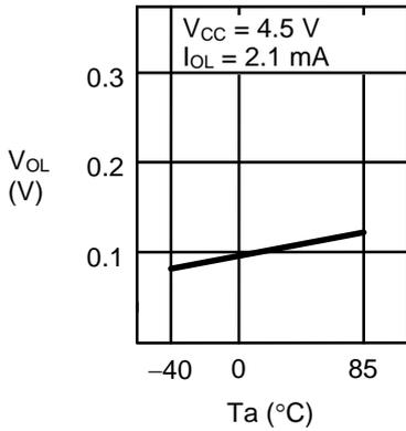
1. 22 Low-level output voltage  $V_{OL}$
