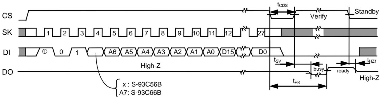
**Figure 11 Data Write Timing (S-93C56B, S-93C66B)**
