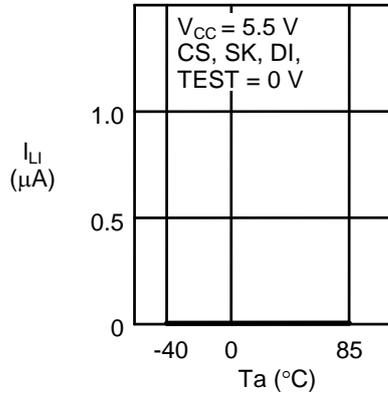
**1. 14 Input leakage current  $I_{LI}$
