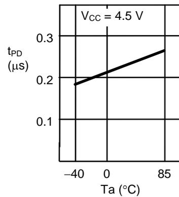
2.7 Data output delay time  $t_{PD}$
