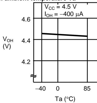
**1. 18 High-level output voltage  $V_{OH}$
