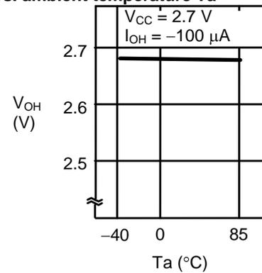
1. 19 High-level output voltage  $V_{OH}$
