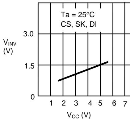
**1. 30 Input inverted voltage  $V_{INV}$
