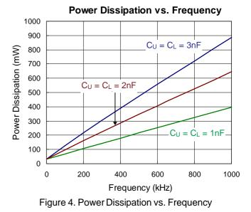
The operating junction temperature can be calculated from the power dissipation curves (Figure 4). Assume  $V_{CC}$  = 12V, operating frequency is 200kHz and  $C_U = C_L = 1nF$  which emulate the input capacitances of the high-side and low-side power MOSFETs. From Figure 4, the power dissipation is  $100m\Omega$ . Thus, for example, with the WDFN-8L 3x3 package thermal resistance  $\theta_{JA}$  is 31°C/W. The operating junction temperature is calculated as :
