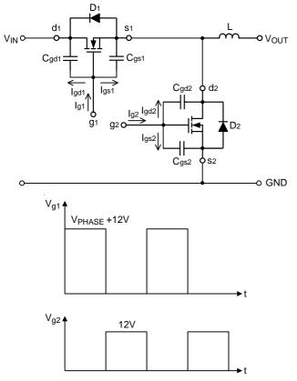
Figure 1. Equivalent Circuit and Associated Waveforms
