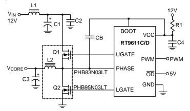
Figure 6. Synchronous Buck Converter Circuit
