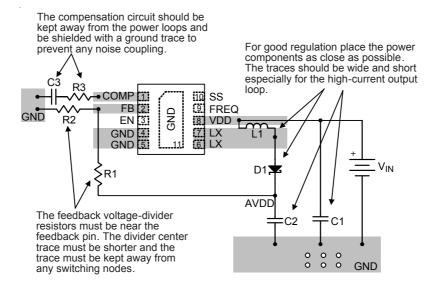
Figure 3. PCB Layout Guide
