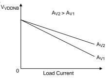
Figure 16. VDDNB Controller : Error Amplifier gain  $(A_V)$ Influence on V<sub>VDDNB</sub> Accuracy
