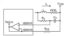
Figure 12. VDD Controller : Lossless Inductor Sensing
