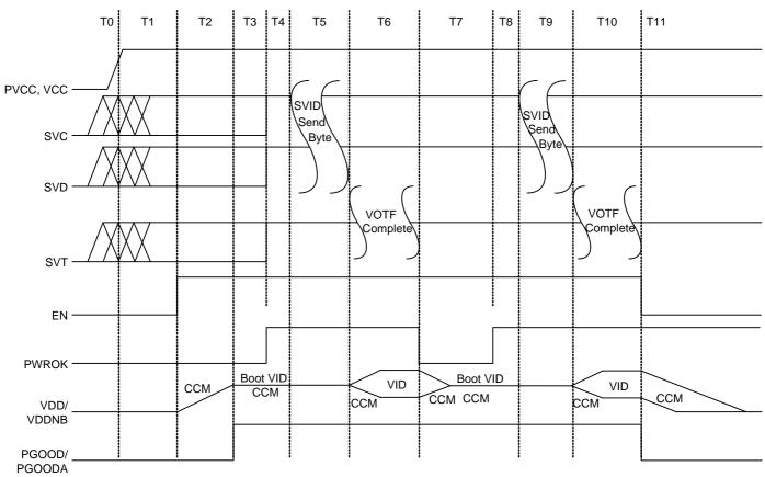
Figure 3. Simplified Sequence Timing Diagram
