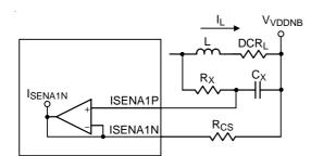
Figure 19. VDDNB Controller : Lossless Inductor Sensing In order to optimize transient performance,  $R_X$  and  $C_X$  must be set according to the equation below :
