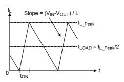
Figure 1. Boundary Condition of CCM/DCM
