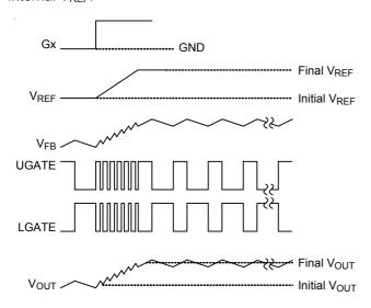
Figure 3. Output Voltage Up Transition
