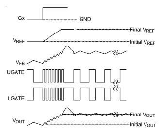
Figure 4. Output Voltage Up Transition with Overshooting
