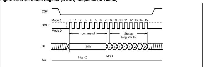
Figure 20. Write Status Register (WRSR) Sequence (SPI Mode)
