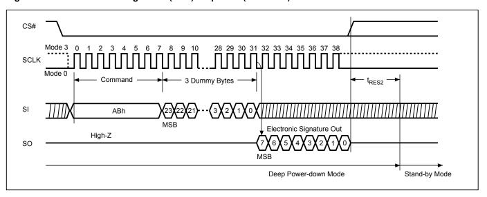
Figure 11. Read Electronic Signature (RES) Sequence (SPI Mode)
