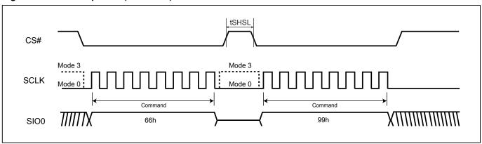
Figure 57. Reset Sequence (QPI mode)
