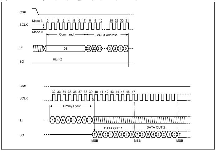
Figure 25. Read at Higher Speed (FAST\_READ) Sequence (QPI Mode)
