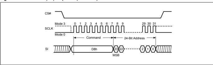
Figure 41. Block Erase (BE) Sequence (QPI Mode)
