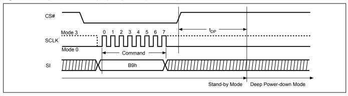
Figure 48. Deep Power-down (DP) Sequence (QPI Mode)
