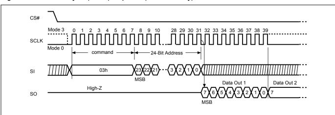
Figure 23. Read Data Bytes (READ) Sequence (SPI Mode only)
