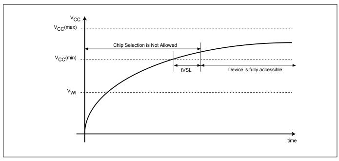
Note: VCC (max.) is 2.0V and VCC (min.) is 1.65V.
