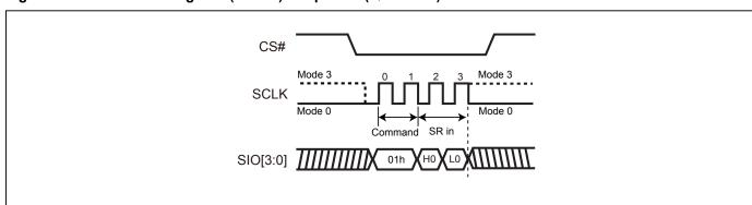
Figure 21. Write Status Register (WRSR) Sequence (QPI Mode)
