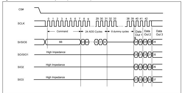
Figure 28. Quad Read Mode Sequence (Command 6B)
