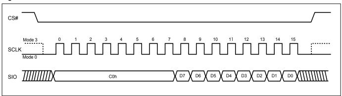
Figure 33. Burst Read - QPI Mode
