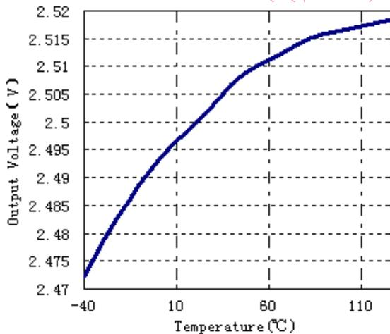
$V_{OUT}=2.5V, I_{LOAD}=1mA, V_{DD}=3.5V$
