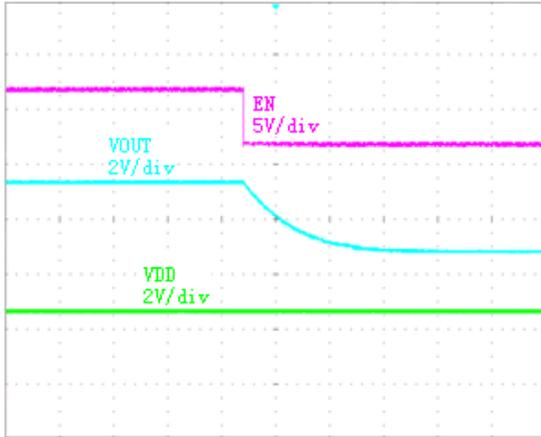
$V_{OUT}=2.5V$ ,  $V_{DD}=3.5$ , no load
