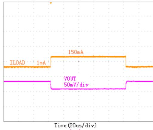
$V_{OUT}=2.5V, I_{LOAD}=10mA, V_{DD}=4.5V \sim 3.5V \sim 4.5V, tr=tf=10\mu s$      $V_{OUT}=2.5V, V_{DD}=3.5V, I_{LOAD}=1mA \sim 150mA \sim 1mA, tr=tf=0.5\mu s$
