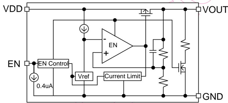
Figure 2(a) Functional diagram of Fix mode
