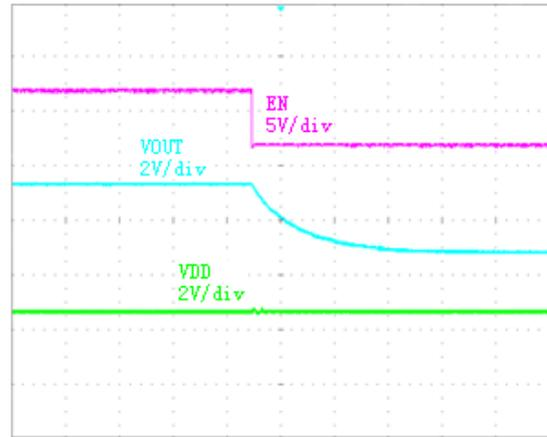
$V_{OUT}=2.5V$ ,  $V_{DD}=3.5$ ,  $I_{LOAD}=50mA$
