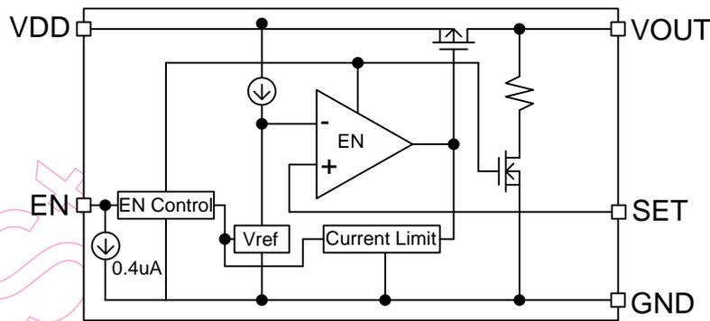
Figure 2(b) Functional diagram of Adjustable mode
