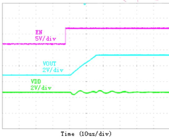
$V_{OUT}=2.5V, V_{DD}=3.5V, I_{LOAD}=0mA$
