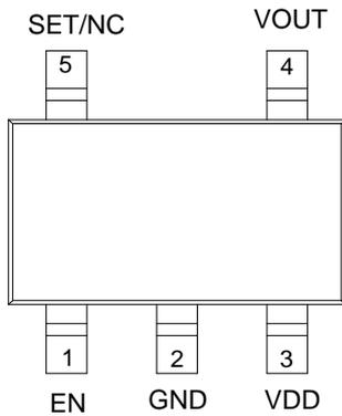
Figure 3d SOT-23-5(S5) package
