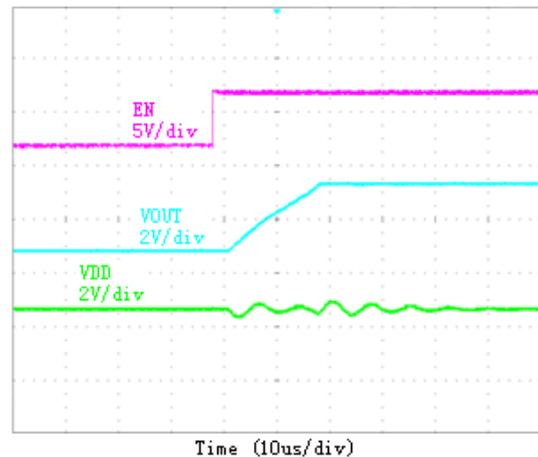
$V_{OUT}=2.5V, V_{DD}=3.5V, I_{LOAD}=50mA$
