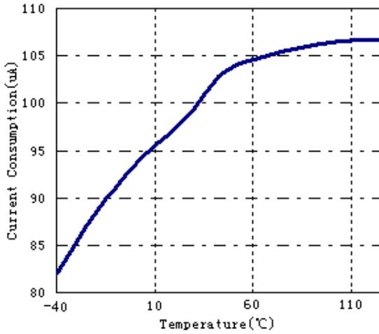
$V_{OUT}=2.5V, V_{DD}=3.5V, I_{LOAD}=0mA$  (FIX)
