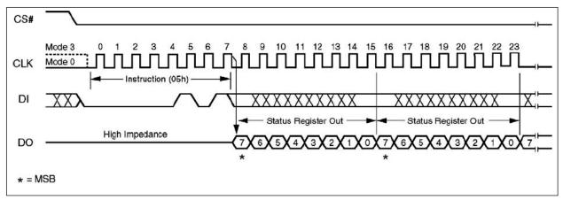
Figure 10. Read Status Register Instruction Sequence Diagram
