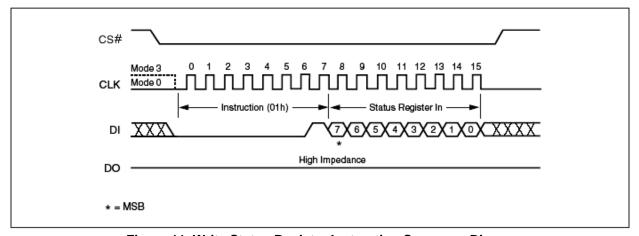
Figure 11. Write Status Register Instruction Sequence Diagram
