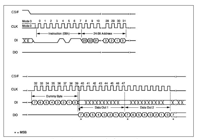
Figure 13. Fast Read Instruction Sequence Diagram
