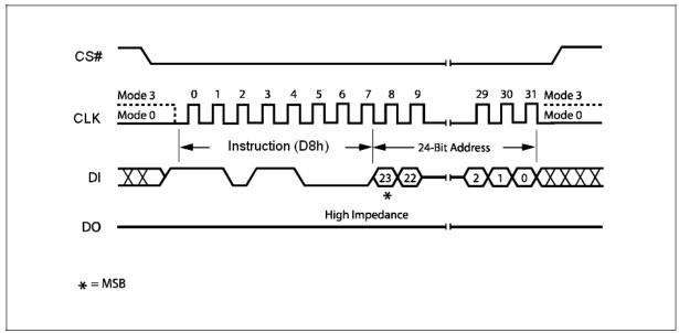
Figure 22. 64KB Block Erase Instruction Sequence Diagram
