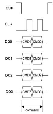
Figure 23.1 Chip Erase Sequence in QPI Mode
