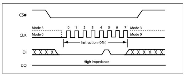
Figure 9. Write Disable Instruction Sequence Diagram
