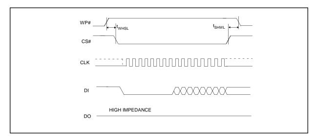
Figure 36. Write Protect setup and hold timing during WRSR when SRP = 1
