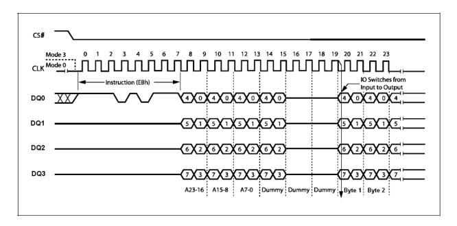
Figure 4. Quad I/O SPI Modes
