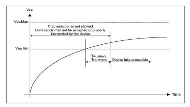
Figure 31. Power-up Timing
