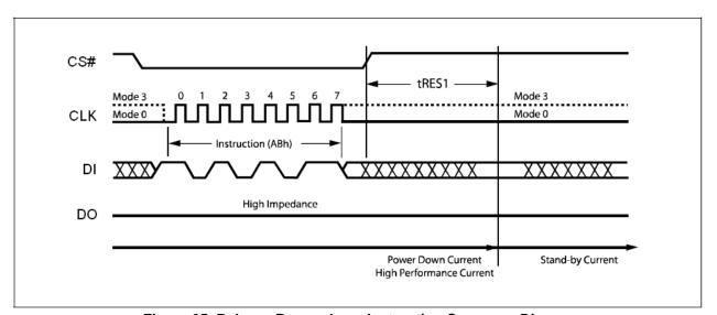
Figure 25. Release Power-down Instruction Sequence Diagram
