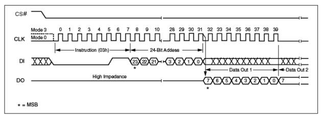
Figure 12. Read Data Instruction Sequence Diagram
