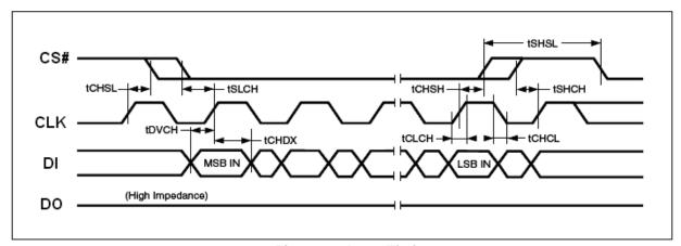
Figure 34. Input Timing
