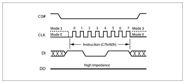
Figure 23. Chip Erase Instruction Sequence Diagram
