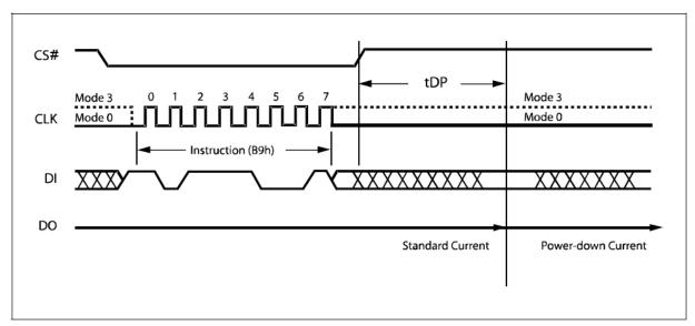
Figure 24. Deep Power-down Instruction Sequence Diagram
