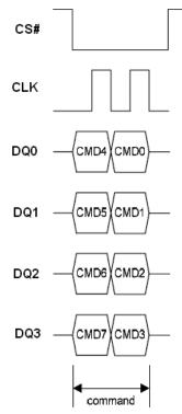
Figure 29.1 Enter OTP mode Sequence in QPI Mode
