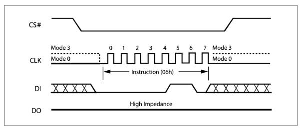
Figure 8. Write Enable Instruction Sequence Diagram
