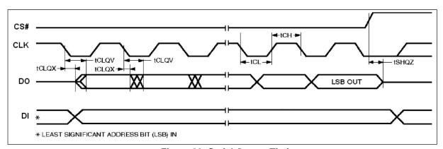
Figure 33. Serial Output Timing
