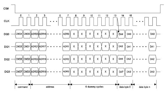
Figure 13.1 Fast Read Instruction Sequence in QPI Mode
