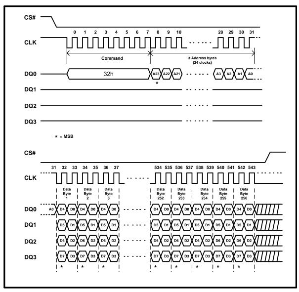
Figure 19. Quad Input Page Program Instruction Sequence Diagram (SPI Mode only)
