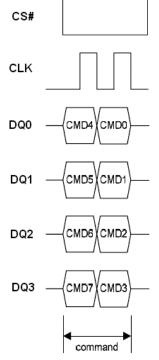
Figure 9.1 Write Enable/Disable Instruction Sequence in QPI Mode
