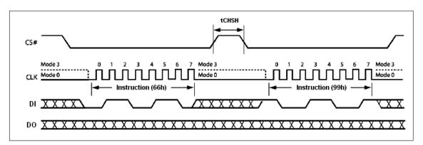
Figure 7. Reset-Enable and Reset Sequence Diagram
