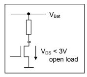
No injection, neither in on-, nor in off-state The engine operates with 3 cylinders, "Limp-home to the workshop" is possible
