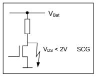
Injection in on- and off-state danger of catalyst damage
