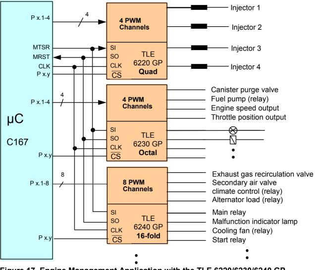
**Figure 17 Engine Management Application with the TLE 6220/6230/6240 GP** rect in parallel for PWM applications.
