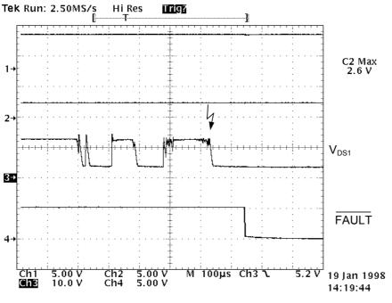
Figure 11 Fault detection via FAULT pin
