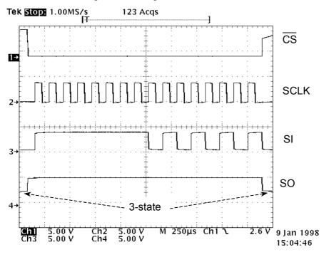
will reset all error registers. Figure 14 shows the TLE 6230 GP controlled by the software tool of evaluation the board. The oscillogram shows the generated signals CS, SCLK, SI and the SO-response of the device. The SO-line indicates normal function for all channels and is tristated before and after CS cycle.
