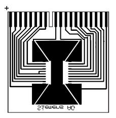
If the devices are mounted on Isolated Metal Substrate (IMS) a thermal resistance of 7 to 10 K/W can be achieved.
