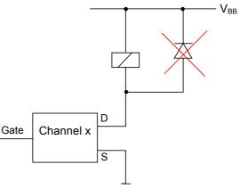
Figure 6 Driving a relay
