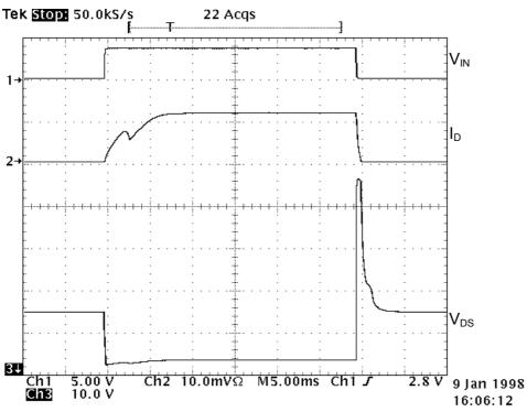
Figure 5 Switching of a Solenoid
