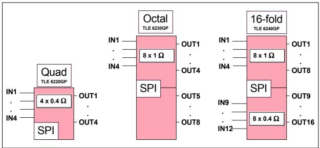
Figure 2 Modular Concept of TLE 62x0 GP Chip Set
