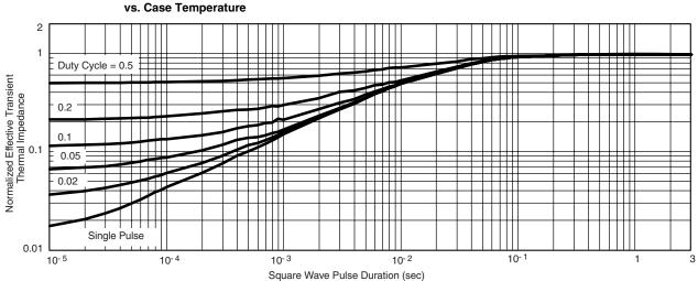
Normalized Thermal Transient Impedance, Junction-to-Case
