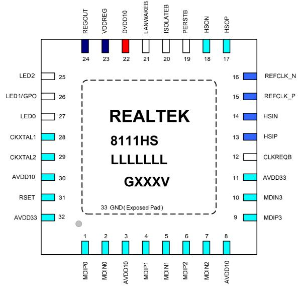
Figure 3. RTL8111HS Pin Assignments
