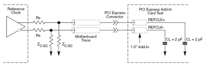
Figure 12. Reference Clock System Measurement Point and Loading
