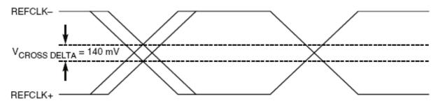
Figure 7. Single-Ended Measurement Points for Delta Cross Point
