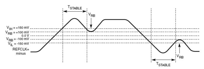
Figure 11. Differential Measurement Points for Ringback
