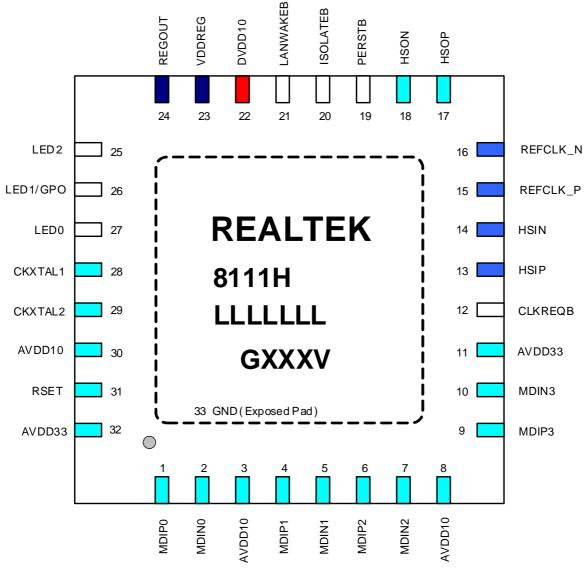
Figure 2. RTL8111H Pin Assignments
