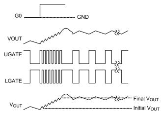
Figure 6. Output Voltage Up Transition with Overshooting
