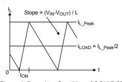
Figure 1. Boundary Condition of CCM/DCM
