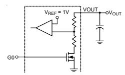
Figure 3. Output Voltage Selection by G0 Input
