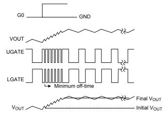
Figure 5. Output Voltage Up Transition
