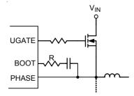
Figure 8. Increasing the UGATE Rise Time
