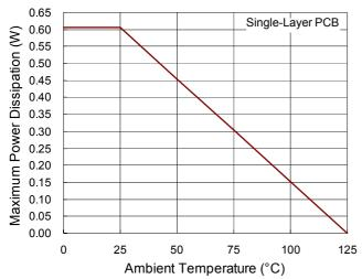
Figure 5. Derating Curves for RT8238A Packages
