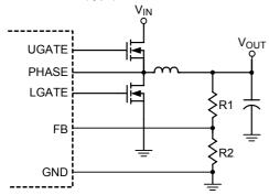
Figure 4. Setting VOUT with a Resistor-Divider
