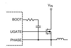
Figure 3. Reducing the UGATE Rise Time
