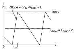
Figure 1. Boundary Condition of CCM/DEM
