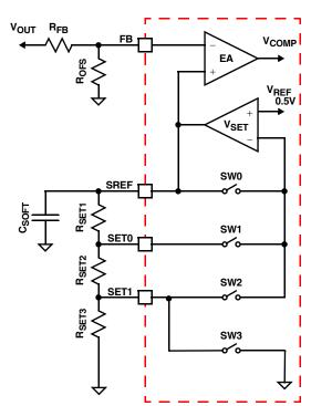
FIGURE 10. ISL95870A VOLTAGE PROGRAMMING CIRCUIT
