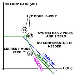
FIGURE 15. UNCOMPENSATED R4 OPEN-LOOP RESPONSE
