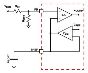
FIGURE 9. ISL95870 VOLTAGE PROGRAMMING CIRCUIT
