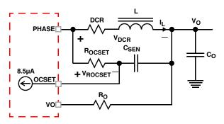
FIGURE 17. OVERCURRENT PROGRAMMING CIRCUIT
