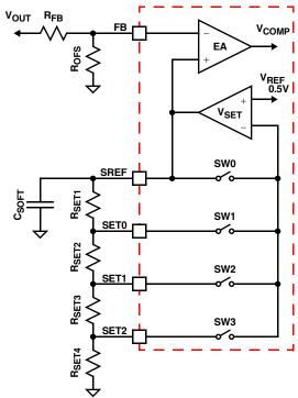
FIGURE 11. ISL95870B VOLTAGE PROGRAMMING CIRCUIT
