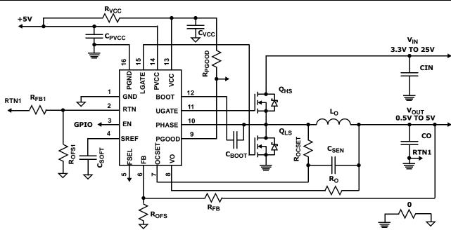
FIGURE 1. ISL95870 APPLICATION SCHEMATIC WITH ONE OUTPUT VOLTAGE SETPOINT AND DCR CURRENT SENSE
