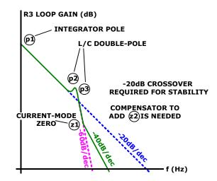
FIGURE 13. UNCOMPENSATED INTEGRATOR OPEN-LOOP RESPONSE
