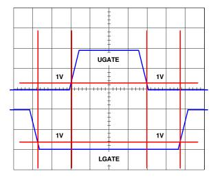
FIGURE 18. GATE DRIVE ADAPTIVE SHOOT-THROUGH **PROTECTION**
