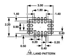
L16.2.6x1.8A 16 LEAD ULTRA THIN QUAD FLAT NO-LEAD PLASTIC PACKAGE
