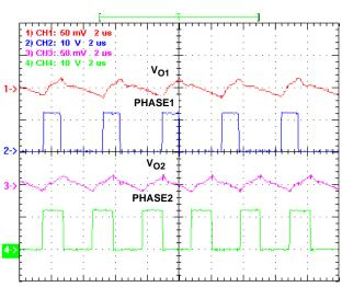
FIGURE 11. CCM STEADY-STATE OPERATION,  $V_{IN}$  = 12V,  $V_{O1}$  = 3.3V,  $I_{O1}$  = 5A,  $V_{O2}$  = 5V,  $I_{O2}$  = 5A
