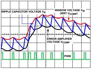
FIGURE 23. MODULATOR WAVEFORMS DURING LOAD TRANSIENT
