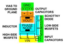
FIGURE 29. TYPICAL POWER COMPONENT PLACEMENT
