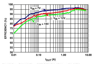
FIGURE 6. CHANNEL 2 EFFICIENCY AT V $_{O}$  = 5V, DEM OPERATION. HIGH-SIDE 1xIRF7821,  $r_{DS(ON)}$  = 9.1m $\Omega$ ; LOW-SIDE 1xIRF7832,  $r_{DS(ON)}$  = 4m $\Omega$ ; L = 4.7 $\mu$ H, DCR = 14.3m $\Omega$ ; CCM  $F_{SW}$  = 330kHz
