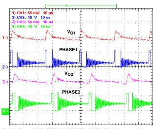
FIGURE 12. DCM STEADY-STATE OPERATION,  $V_{IN}$  = 12V,  $V_{O1}$  = 3.3V,  $I_{O1}$  = 0. 2A,  $V_{O2}$  = 5V,  $I_{O2}$  = 0. 2A
