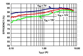
FIGURE 5. CHANNEL 1 EFFICIENCY AT V $_{O}$  = 3.3V, DEM OPERATION. HIGH-SIDE 1xIRF7821,  $r_{DS(ON)}$  = 9.1m $\Omega$ ; LOW-SIDE 1xIRF7832,  $r_{DS(ON)}$  = 4m $\Omega$ ; L = 4.7 $\mu$ H, DCR = 14.3m $\Omega$ ; CCM  $F_{SW}$  = 270kHz
