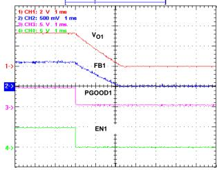
FIGURE 10. ENABLE CONTROL, EN1 = LOW,  $V_{\text{IN}} = 12V$ ,  $V_{\text{O}} = 3.3V$ ,  $I_{\text{O}} = 5A$
