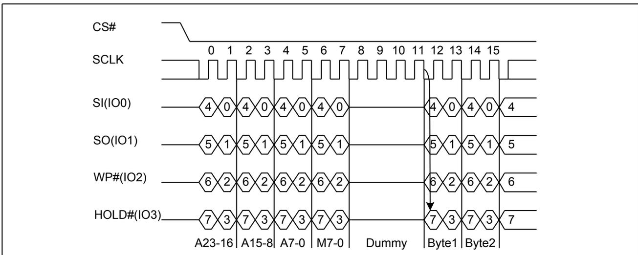
**Quad I/O Fast Read with “8/16/32/64-Byte Wrap Around” in Standard SPI Mode**
