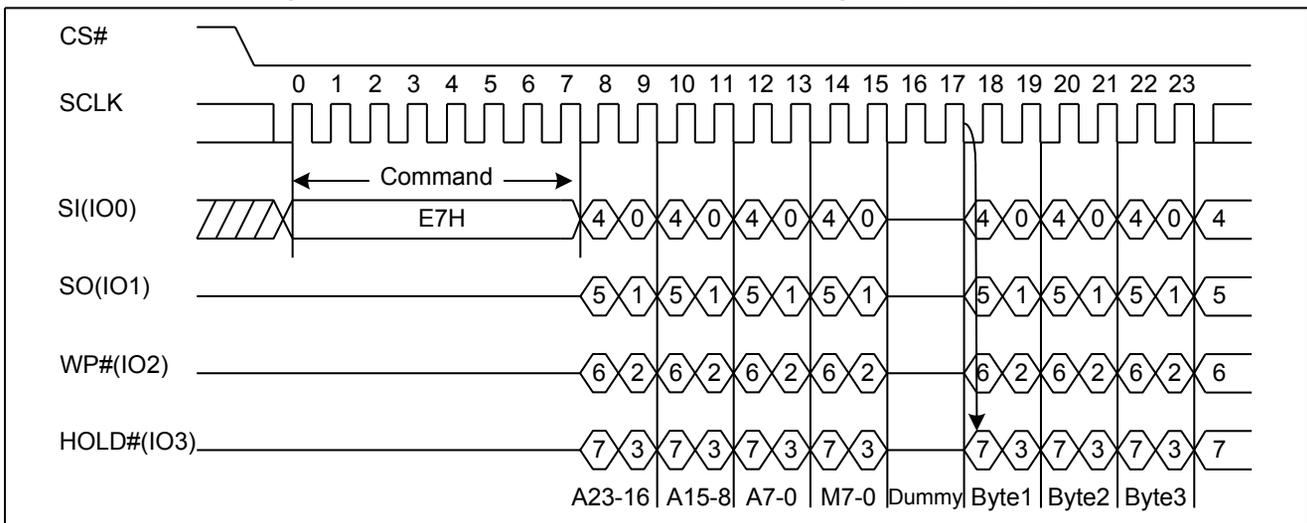
**Figure14a. Quad I/O Word Fast Read Sequence Diagram (M5-4= (1, 0))**
