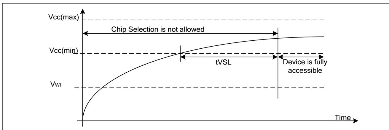
Table 8.1. Power-Up Timing and Write Inhibit Threshold
