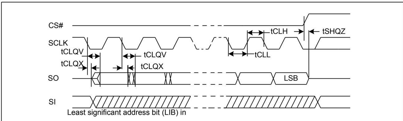
Figure47. Resume to Suspend Timing Diagram
