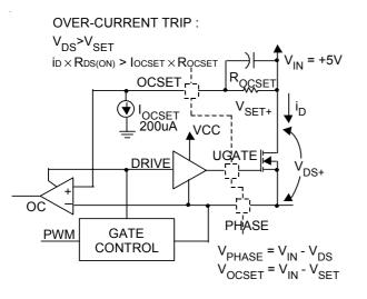
Figure 6. Current Limiting Setting
