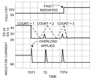
Figure 5. Over-current Operation
