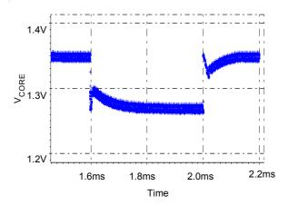
Figure 14. V<sub>CORE</sub> Wave Form at Load Transient
