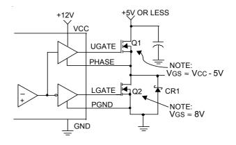
Figure 15. Upper Gate Drive-direct V<sub>CC</sub> Drive
