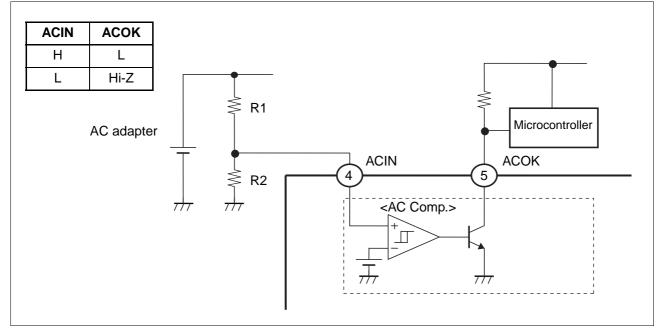
AC adapter detection voltage setting
